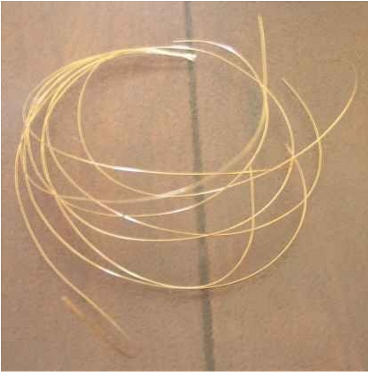
Form one of the longest wires into a loop and attach (wrap the loose end) it to the base where all the wires are twisted together
